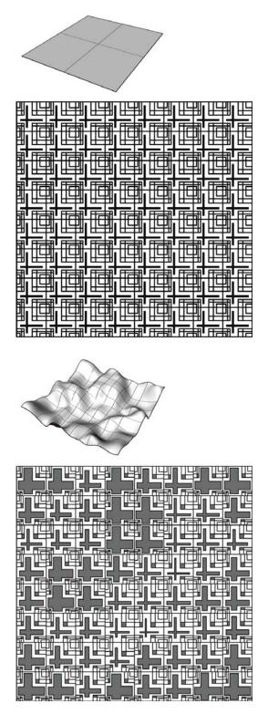
Figure 4: Pattern Variation through external controlled input. The relative height of the surface determines the degree of opening within the pattern
