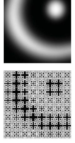
Figure 5: Pattern Variation through external control input. The value of the image determines the opening of the pattern at each point
