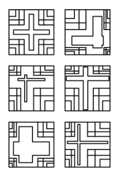
Figure 3: Original Frank Lloyd Wright design of the Millard House textile block and new designs from parametric variations.
